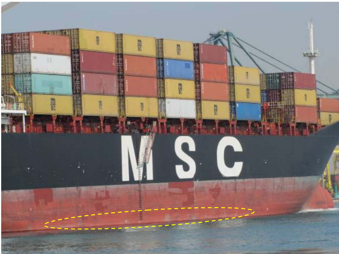
Figure 7 – MSC ELOISE light scratches on parallel body
