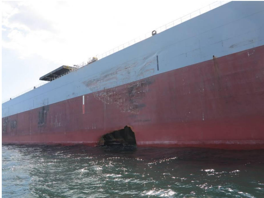
Figure 7.3/7.4 – CAPE MED damage on the port side
