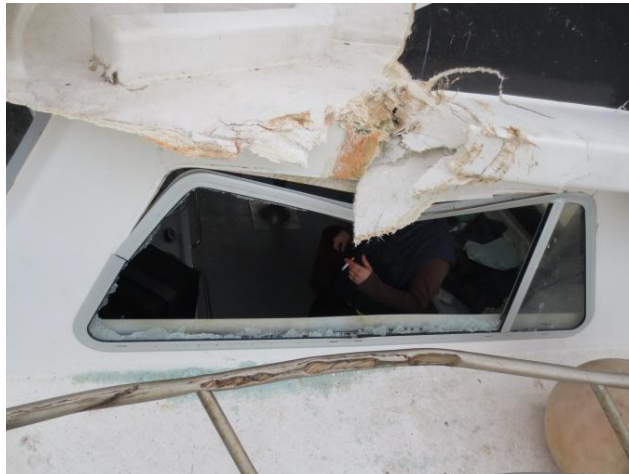
Figure 5.4–Damages on Port side bridge
