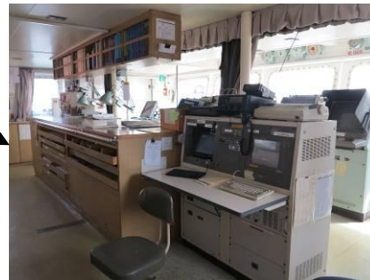
Figure 2.2- TERVE Bridge arrangements
