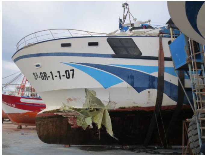
Figure 5.1– Hull Damages on Port side
