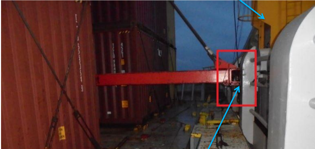
Point of fatal strike between spreader and ship's construction
