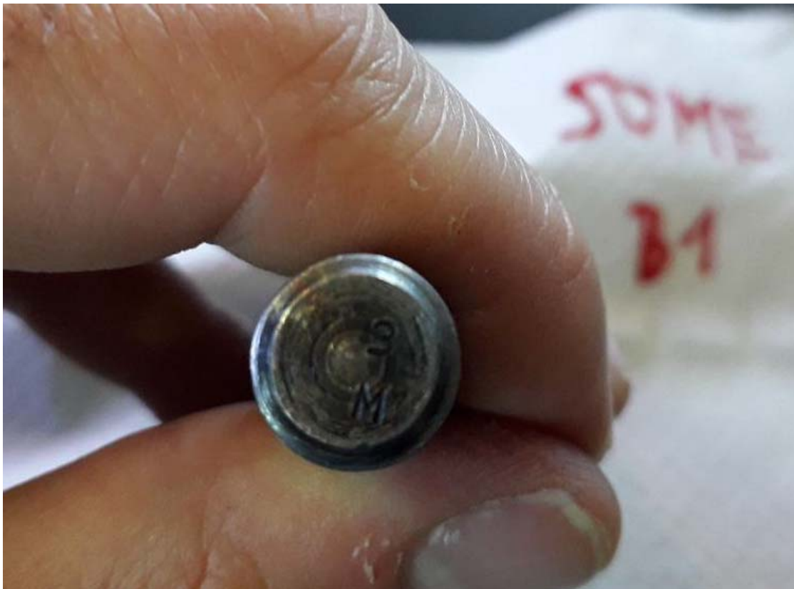
Figure 10. VOLCAN DE TENO. One of the new-design studs, stamped with a "3"
