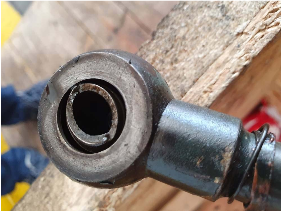
Figure 9. VOLCAN DE TENO. Broken fuel line "banjo bolt"
