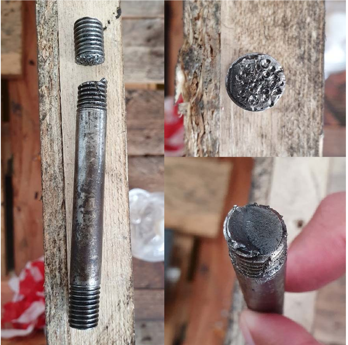
Figure 11. VOLCAN DE TENO. One of the snapped studs
