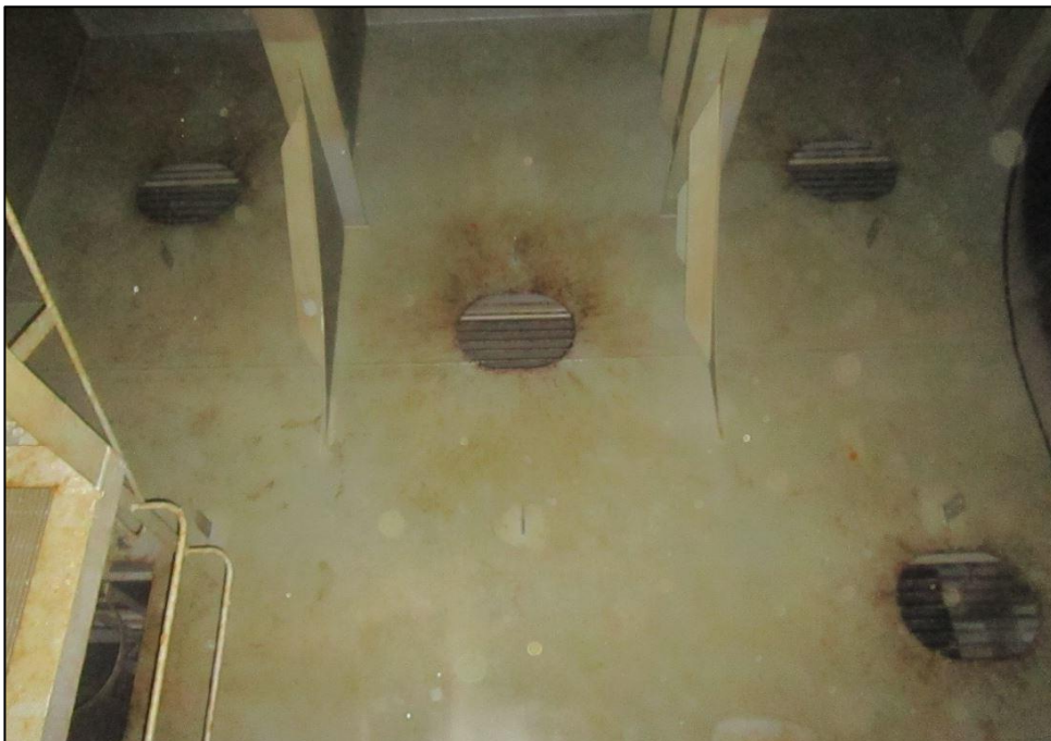
Figure 16: Protected openings on tween decks of other water ballast tanks
