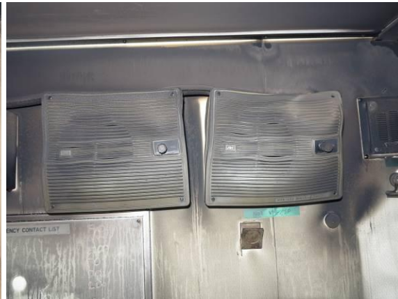
Figure 8.7 – Melting of speakers in Captain office
