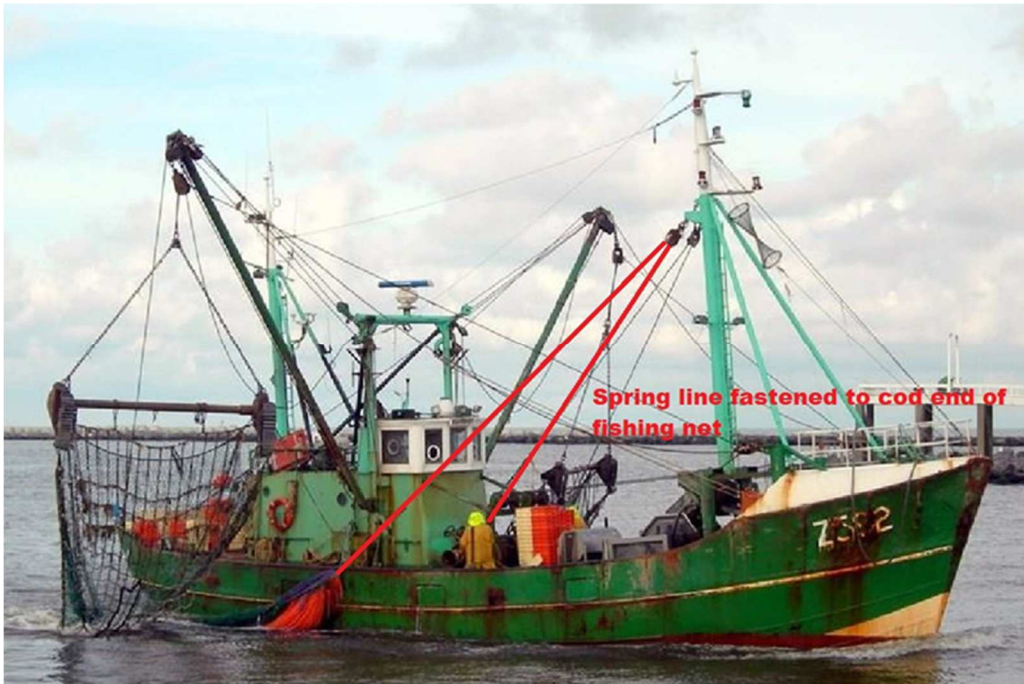
Figure 35 – spring line (coloured red) fastened to starboard fishing net on board the Z582 ASSANAT archive picture)
