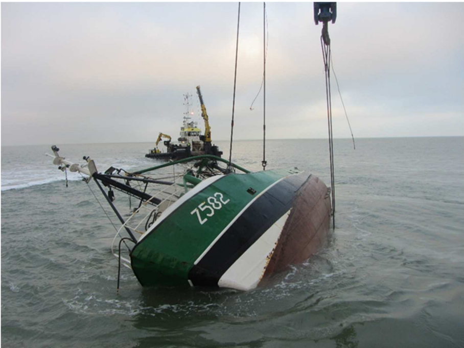
Figure 7 – Z582 ASSANAT Being turned right side up
