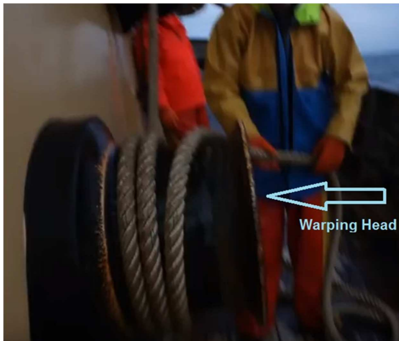
Figure 36 - Running a spring line over a turning warping head of a winch
