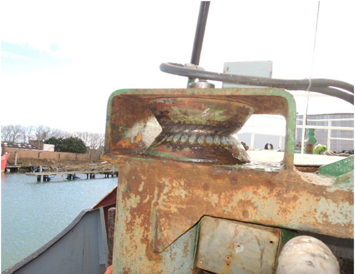
Figure 18 - fairlead through which the net warp was rigged equipped with hydraulics to measure line length of the warp and forces on the warp
