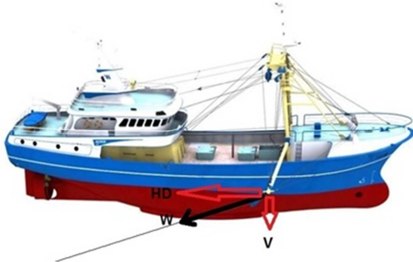
Figure 22 – Pictorial representation of components of the force on the end of the boom when beam trawling
