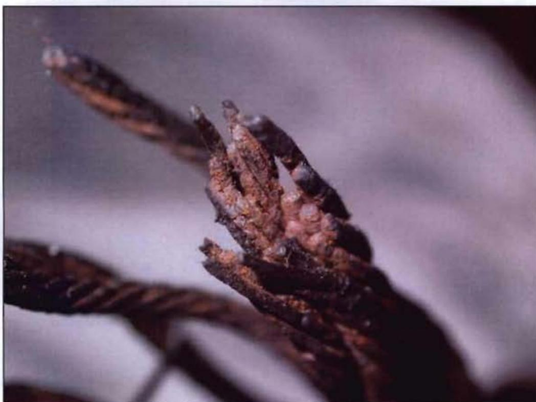
**Figure 17: Close up of inner strands showing advanced corrosion**
