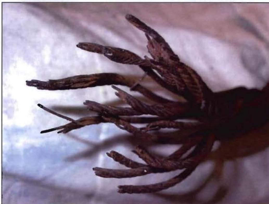
**Figure 16: Inner strands of the wire rope**
