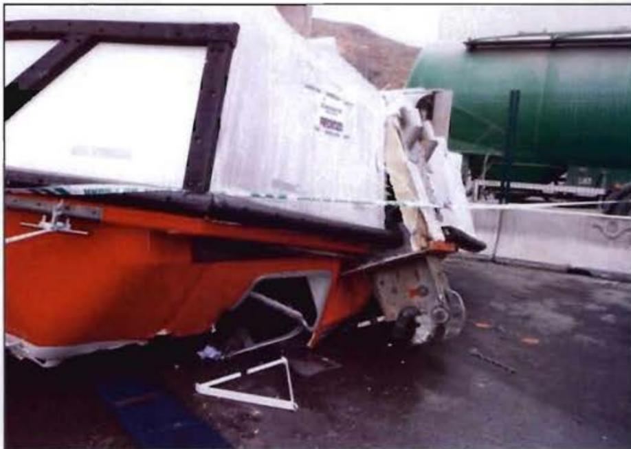
**Figure 12: Damage to aft end of lifeboat tender no. 9**
