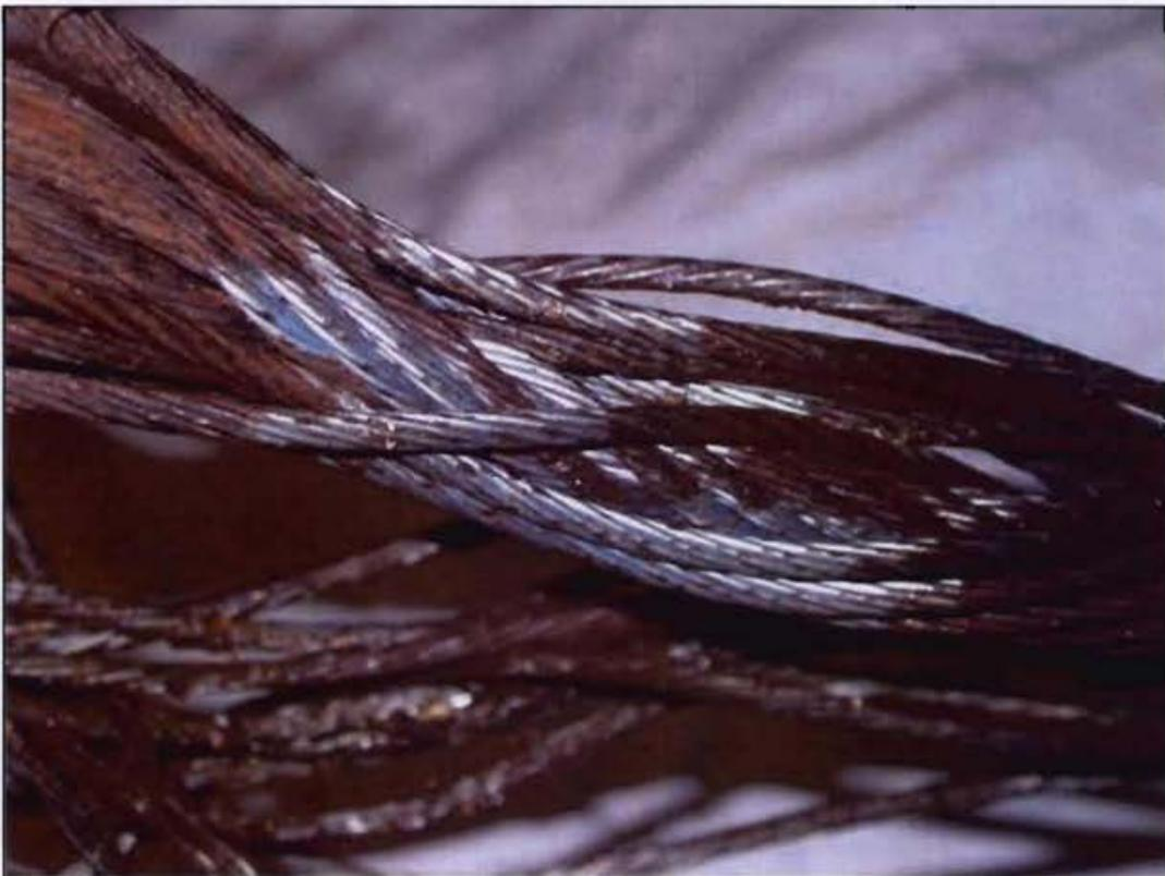
**Figure 15: Evidence of residual galvanization**
