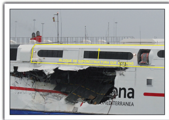
Figure 17. Superstructure block of vessel MILENIUM DOS that was raised
