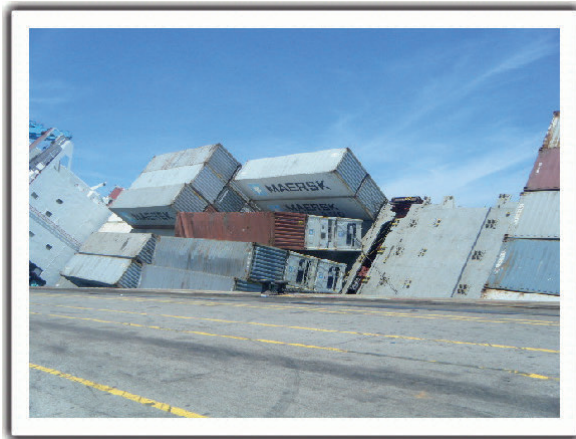
Figure 7. Containers over bay 2, whose locking mechanisms did not withstand the heeling
