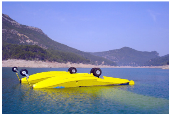
Figure 24. A-019/2012 - Condition of the aircraft after the accident
