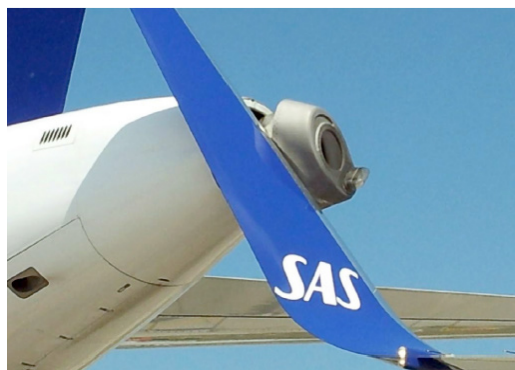
Figure 13. IN-033/2011 - Close-up of the B-737 winglet lodged against the APU exhaust nozzle on the A-320
