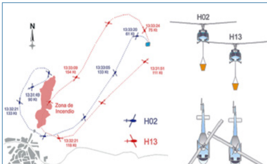
Figure 15. A-037/2011 - Flight paths before the impact and positions of aircraft just before the first blade impacted
