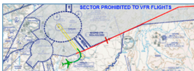
Figure 8. IN-040/2010 - Flightpaths of EC-FAN (red) and EC-HDK (green)
