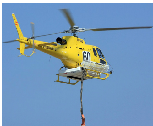
Figure 29. A-032/2012 - Helicopter and the Simplex 310 firefighting system
